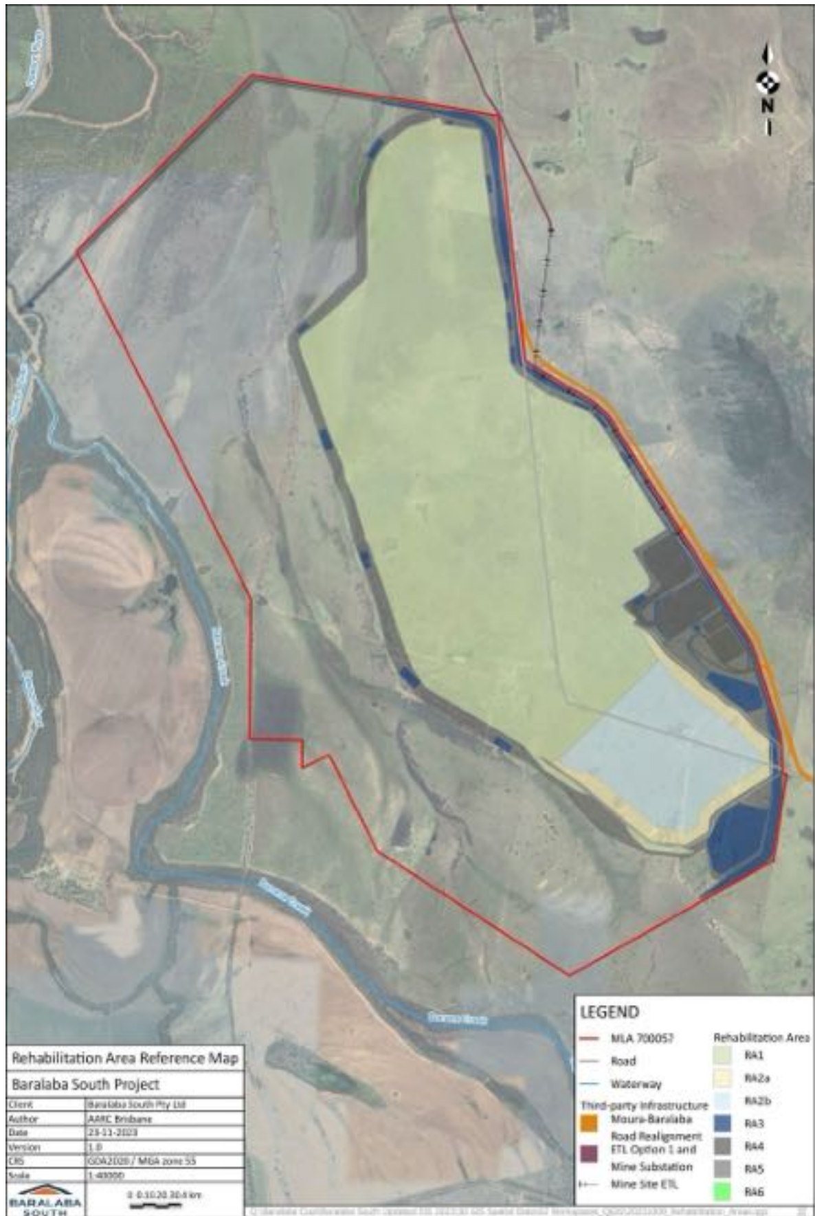
Figure 29: Rehabilitation area reference map
