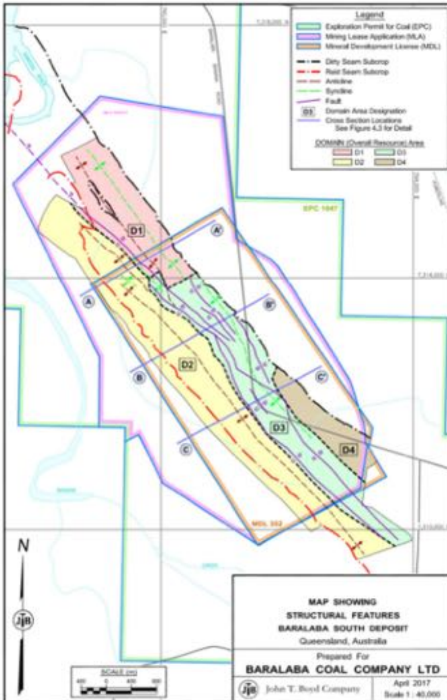
Figure 2-11 Seam Sub-crop and Section Plan at MLA 700057 [source: John T Boyd Company, 2017]
