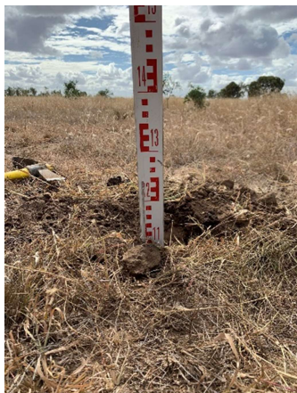
5. Hydraulic permeability testing at BH03.
