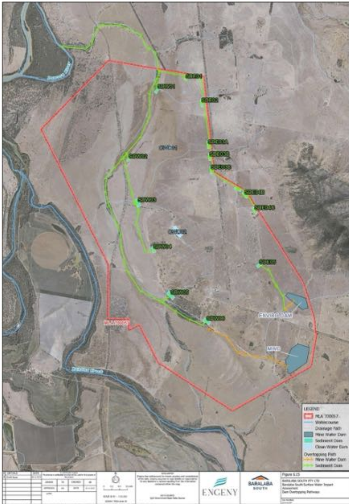
Figure 9.29: Overflow pathways for water management infrastructure
